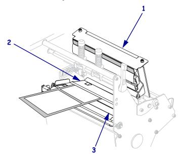
**9.** Extend approximately 36 in. (920 mm) of media out of the printer. Remove and discard the labels from this exposed media.
